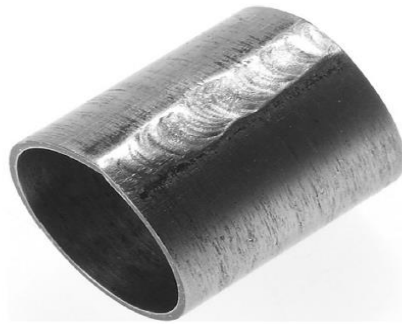
Fig. 2.4: Finished prototype Fe-SMA coupling [42][43]
