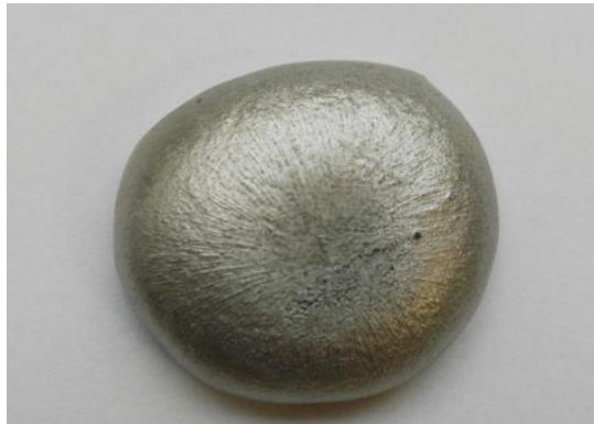
Fig. 4.3: Fe-15Mn-10Cr-8Ni-4Si (wt. %) Fe-SMA button
