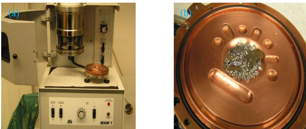
Fig. 4.2: (a) Arc melting machine and (b) copper crucible plate
