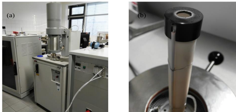
Fig. 4.10: (a) Netzsch LFA 427 apparatus and (b) specimen holder having specimen along with a thermocouple
