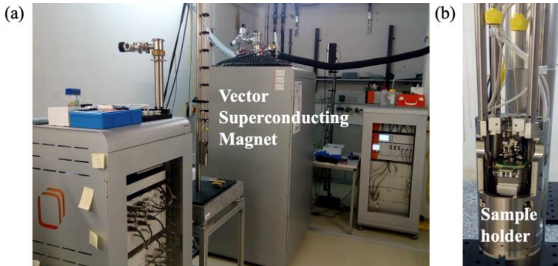
Figure 1.13 MFM setup with model AttoLiquid MFMF I from the company Attocube. (a) Chambers for low temperature measurement and superconductor vector magnet and (b) Sample holder with the magnetic tip and piezo stage.
