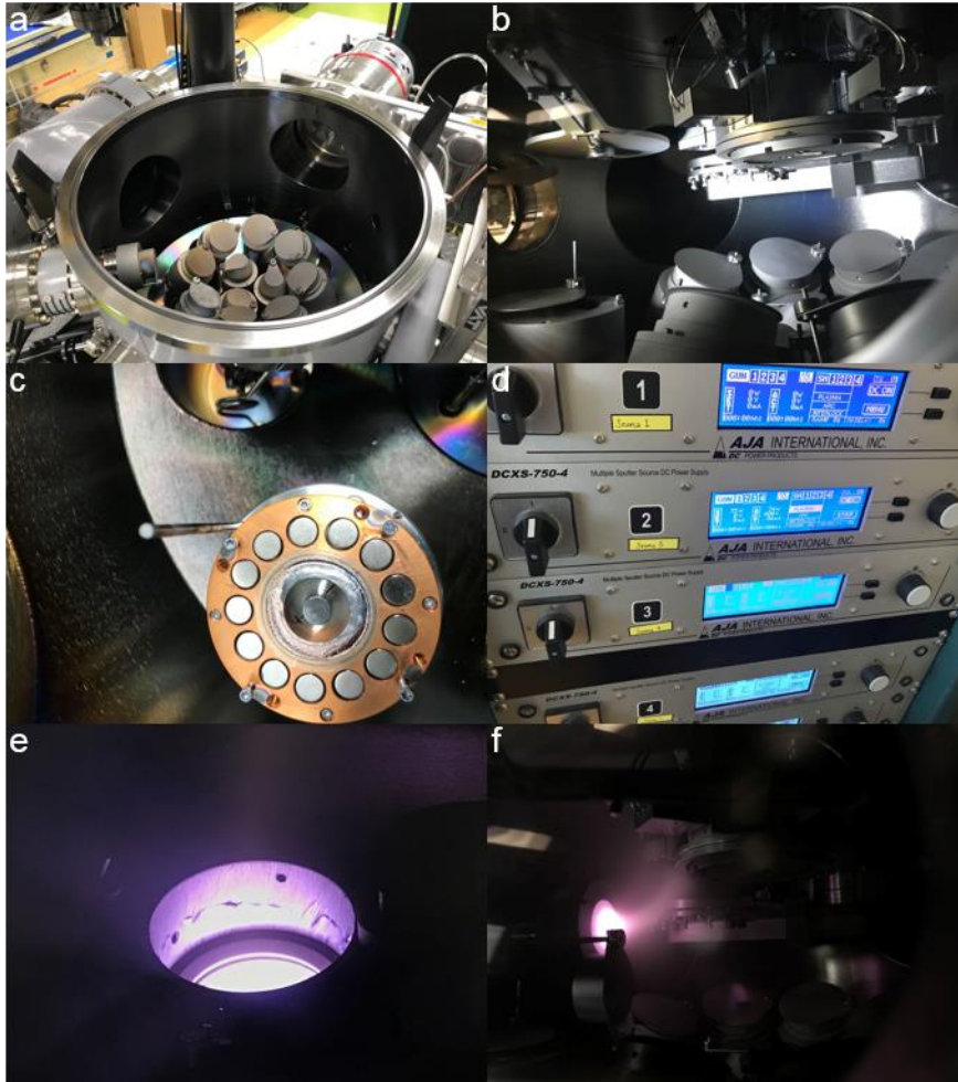
Figure 1.1 (a) - (f) Magnetron sputtering equipment and process of sputtering.
