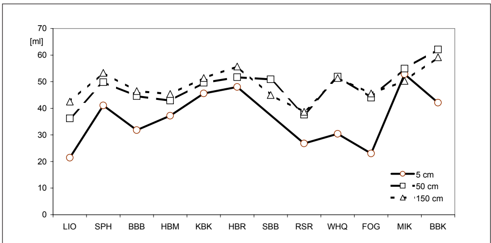
Fig. 9 Piche evaporation measured at different heights on the one-day measurement campaign on July 20, 1995 and summed up from 5 am until 5 pm. For site abbreviation see Fig. 1. Sites are arranged from west (LIO) to east (BBK).
