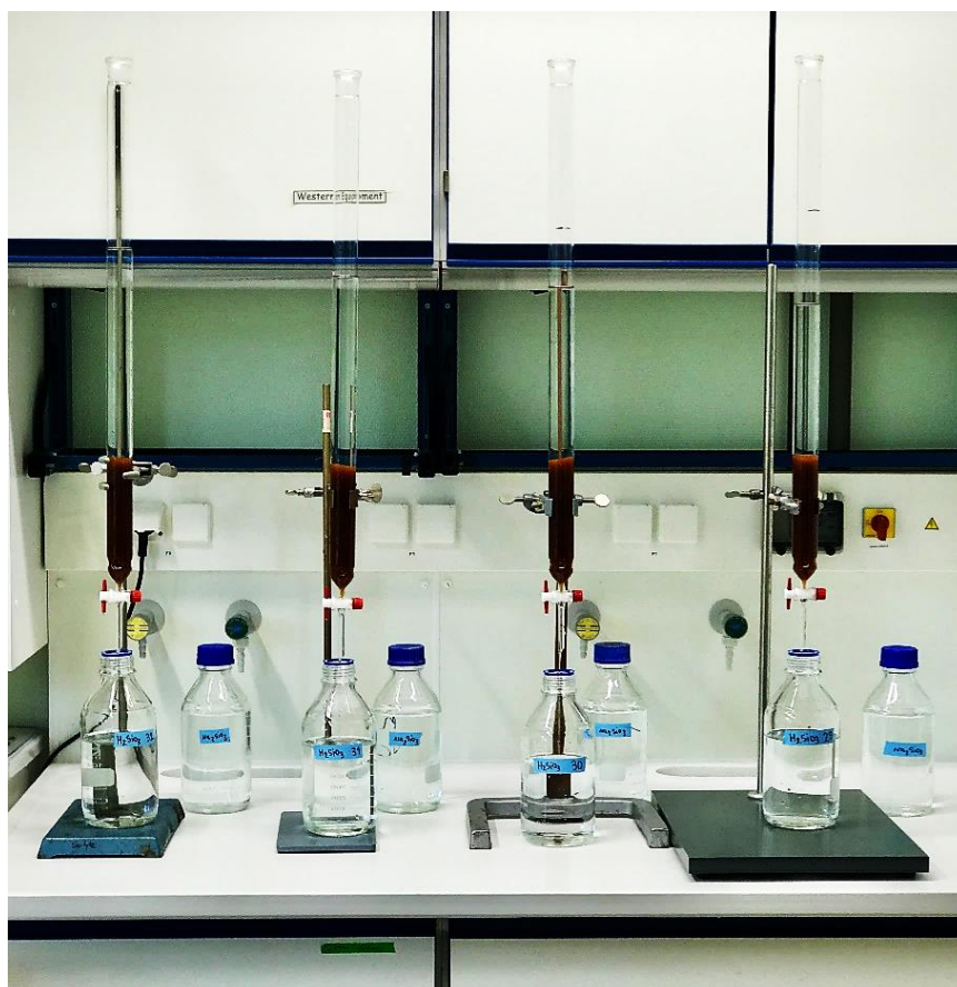
Figure 4. Preparing monosilicic acid ( \text{H}_2\text{SiO}_4 ) from sodium metasilicate nonahydrate ( \text{Na}_2\text{O}_3\text{Si}\cdot 9\text{H}_2\text{O} ) by column chromatography. The column was filled with amberlite that adsorbed sodium through the cation exchange process.
