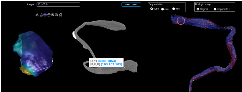
Figure 7.10: Visual exploration of combined microCT and histology; left: 3D model with WSS, white line indicates the current slice; middle: segmented microCT image, right: segmented, corresponding MT-stained histologic image
