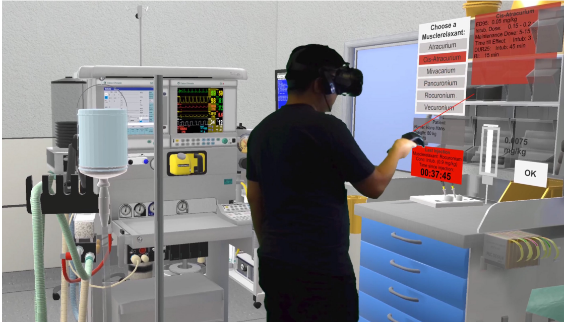
FIGURE 5.5: An example of interactions for choosing different muscle relaxant medications. A user is captured using a chroma keying technique and a green screen to embed in the virtual environment to demonstrate how the user interacts in VR.
