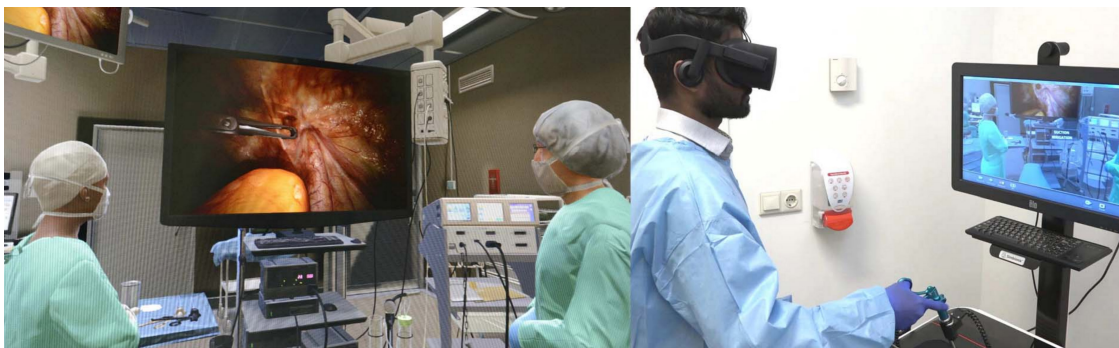
FIGURE 3.2: The setup of the laparoscopic simulation in the virtual operating room with virtual assistants: replicated operating room surrounding in VR (left) and an external view of a surgical trainee in the physical world (right). Figure from Li et al. [78] ©2020 IEEE.
