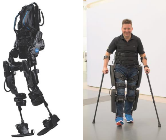
Figure 18: Left: EksoNR™ (Ekso Bionics, Richmond, USA) Right: ReWalk (ReWalk Robotics, Yokneam, Israel)
