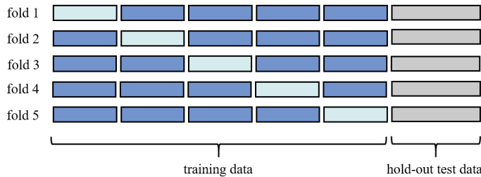
Figure 2.17: Exemplary k -fold cross validation ( k = 5 ) where the turquoise boxes represent the validation samples for the network training.
