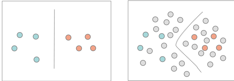
Figure 2.14: Illustration of the modification in the hypothesis or the decision boundary under the influence of unlabeled data. The left image portrays the decision boundary when using only labeled data, where turquoise circles belong to class A and red circles to class B. The right image portrays the change in decision boundary under the influence of unlabeled data denoted by grey circles.
