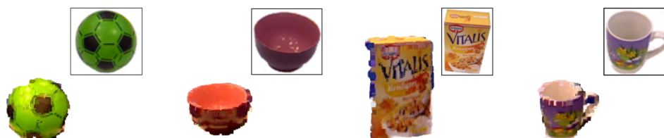
Figure 2.8: RoCS dataset samples: Point cloud and RGB images of a ball , bowl , paper box , and cup (for visualization purposes, images are scaled and 3D points are magnified).
