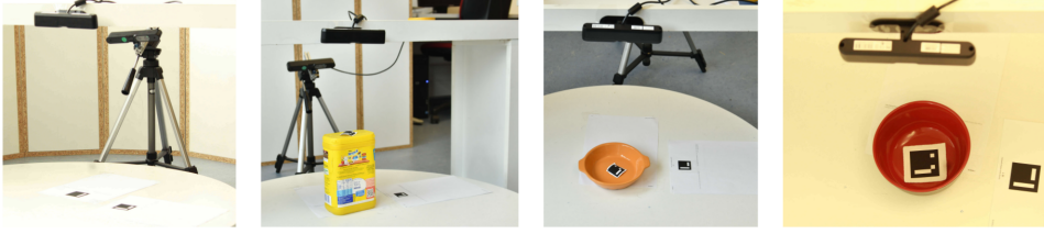
Figure 2.5: Light-weight experimental setup consisting of two cameras and fiducial markers [41], for acquiring physical properties.
