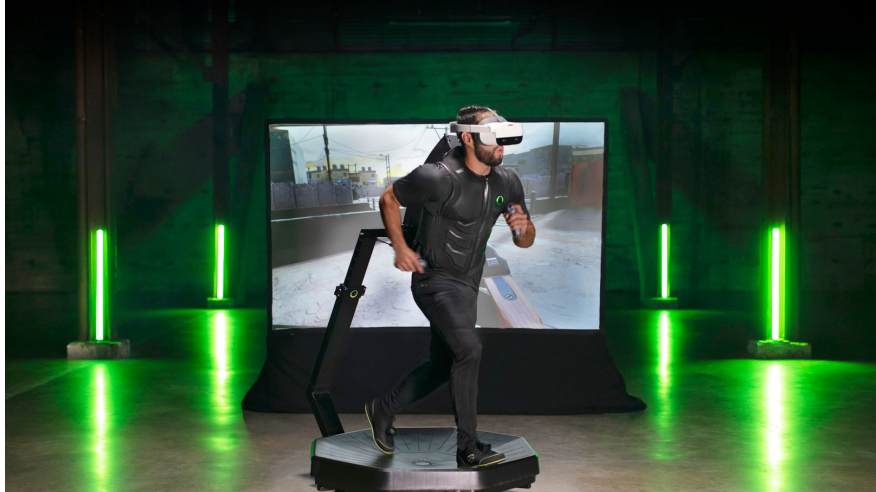
Figure 2.7: Image of a commercial omni-directional treadmill developed for VR. Image from Omni One by Virtuix [67].
