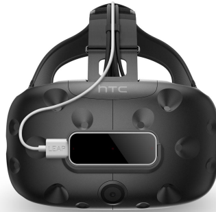
Figure 2.6: Leap Motion mounted on a HTC Vive. Image from [62].
