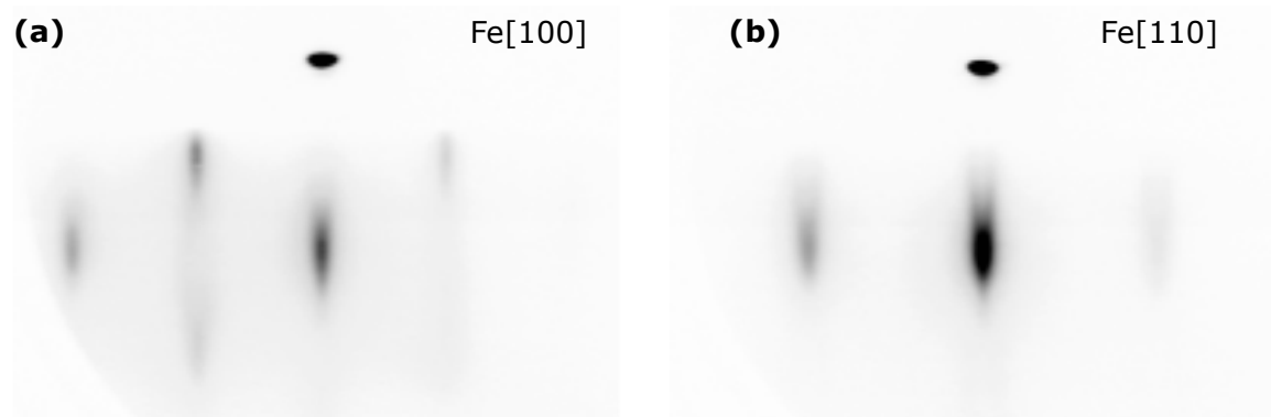
Figure 6.3.: RHEED pattern of the 10 nm thick Fe seed layer where the electron beam is oriented along the (a) [100] and (b) [110] direction.
