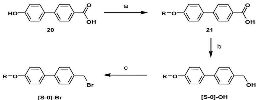
**Scheme 3.9** Preparation of the **S** mesogenic unit **[S-o]-Br**. **R** = CH<sub>3</sub>-(CH<sub>2</sub>)<sub>11</sub>- (a) 1-bromo-dodecane, KOH, EtOH/water, reflux, (b) LiAlH<sub>4</sub>, THF, reflux, 71 % over two steps, (c) CBr<sub>4</sub>, PPh<sub>3</sub>, THF, RT, 85 %.
