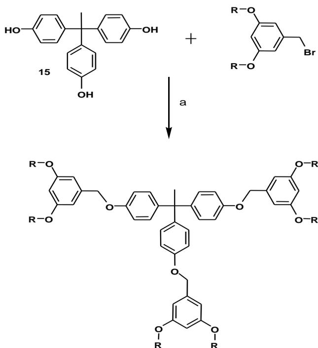
**Scheme 3.3** Attachment of dendrons to the core unit (a)  $K_2CO_3$ , 18-crown[6], acetone (and occasionally THF).
