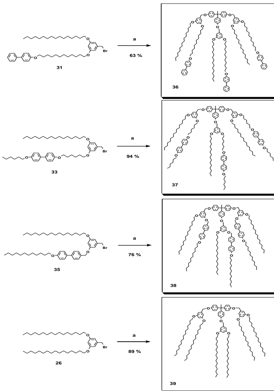
**Scheme 3.19** Formation of the first generational dendrimers. (a) **15**,  $K_2CO_3$ , 18-crown[6], acetone, reflux
