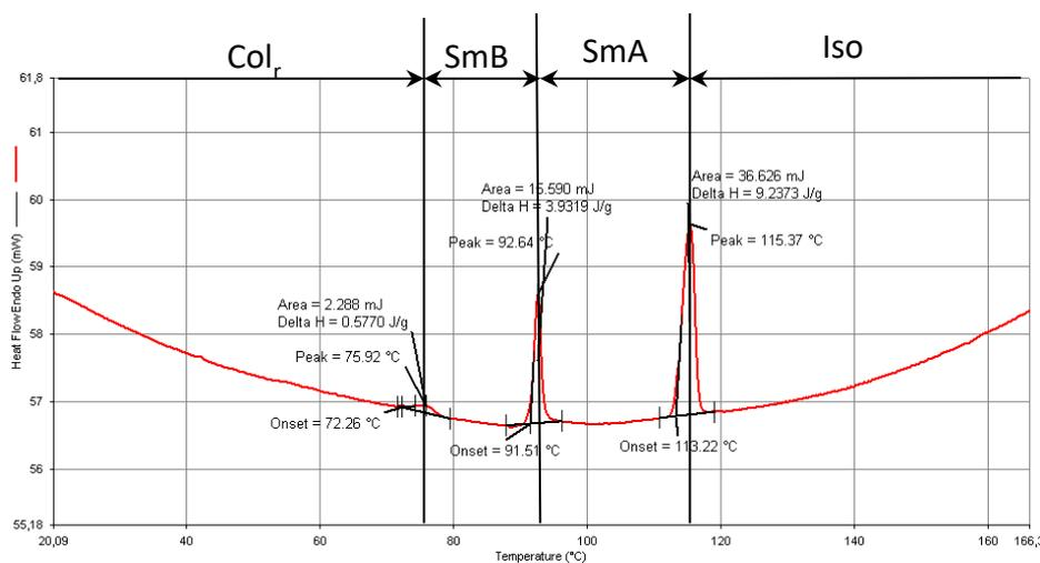
**Figure 4.4** Differential scanning calorimetric curve of [M-2]-C. Second heating (10 K min<sup>-1</sup>).
