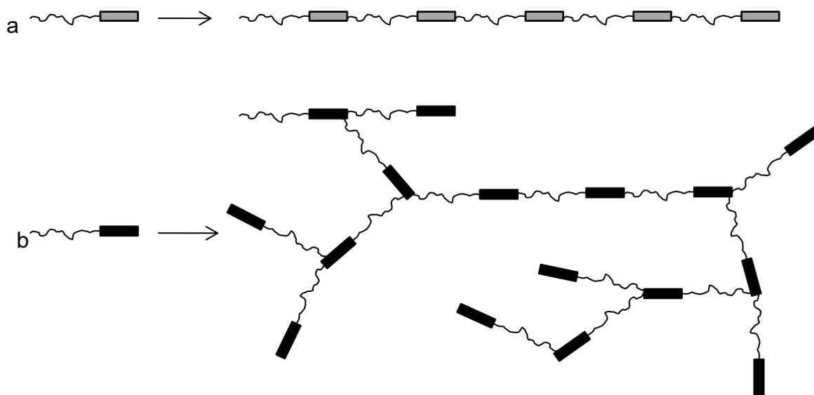
**Figure 1.7** Schematic representation of a main-chain LC polymer (a) and a hyperbranched LC polymer (b)
