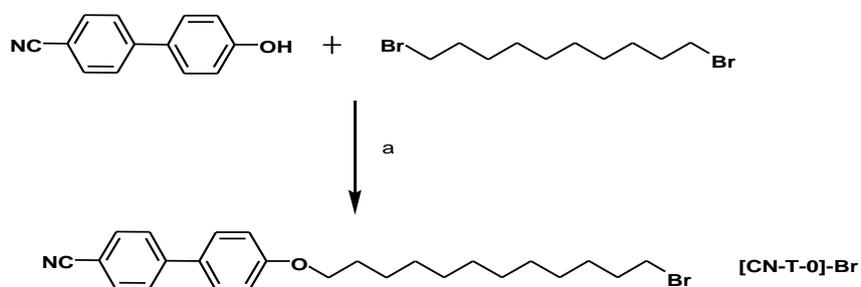
**Scheme 3.5** Synthesis of **CN-T** mesogenic unit. (a) DMF,  $K_2CO_3$ , RT, 81 %.
