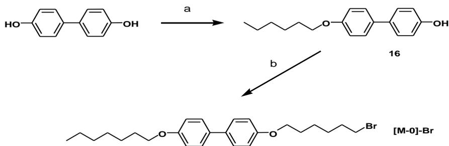
**Scheme 3.6** Synthesis of the **M** mesogenic unit. (a) 1-bromo-hexane, NaOH, EtOH, reflux, 78 %, (b) Br-(CH<sub>2</sub>)<sub>6</sub>-Br, DMF, K<sub>2</sub>CO<sub>3</sub>, RT, 79 %.
