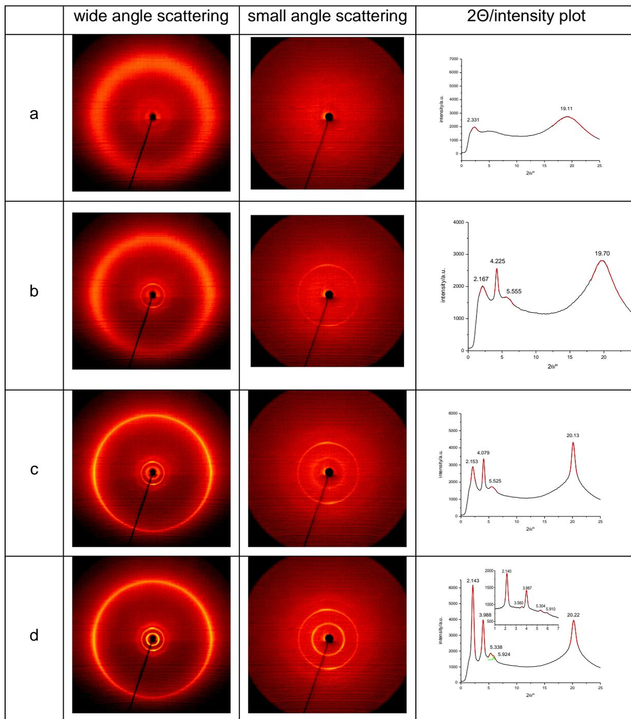
**Figure 4.5** X-ray diffraction patterns of [M-2]-C at different mesophases. a, 120 °C, isotropic liquid, b, 100 °C, smectic A phase, c, 80 °C, smectic B phase, d, 60 °C, rectangular columnar phase
