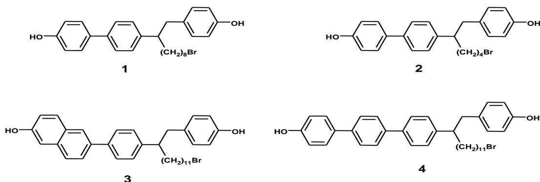
**Figure 1.8** Monomers used to create hyperbranched polymeric LCs
