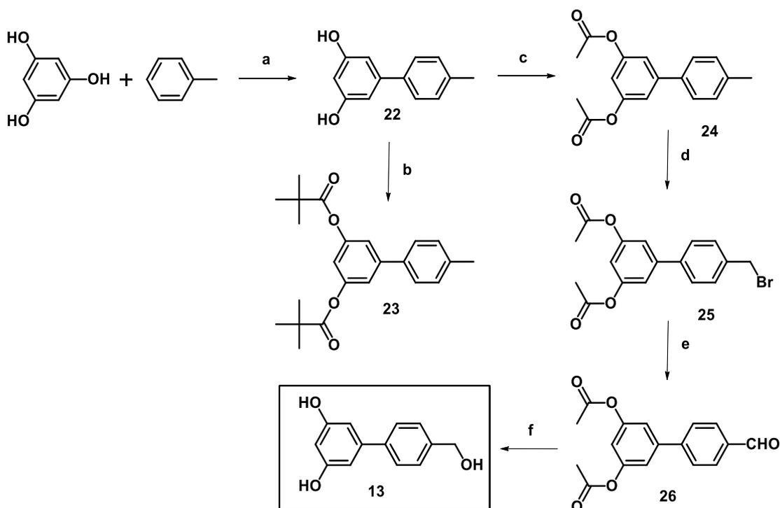
**Scheme 3.16** Reaction route towards the 4-(3,5-dihydroxyphenyl)-benzyl alcohol. (a)  $\text{AlCl}_3$ , RT, 70 %, (b) pivaloyl chloride, pyridine, ice-cooling  $\rightarrow$  60 °C, 46 %, (c)  $(\text{CH}_3\text{CO})_2\text{O}$ , pyridine, RT, 85 %, (d) N-bromo-succinimide,  $\text{CCl}_4$ , benzoyl peroxyde, reflux, 76 %, (e)  $\text{CH}_3\text{COONa}$ , DMSO, 70 °C, 85 %, (f)  $\text{LiAlH}_4$ , THF, reflux, 92 %.
