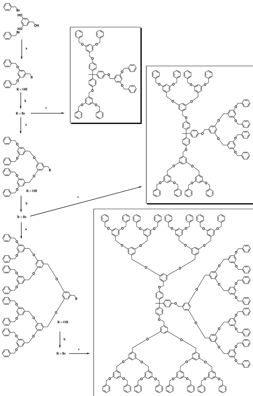
**Scheme 3.2** Overview of the synthetic path to the Fréchet-type dendrons and dendrimers. (a) 3,5-dihydroxybenzyl alcohol,  $K_2CO_3$ , 18-crown[6], acetone, reflux, (b)  $CBr_4$ ,  $PPh_3$ , THF, RT, (c) 1,1,1-tris(4-hydroxyphenyl)ethane,  $K_2CO_3$ , 18-crown[6], acetone, reflux.
