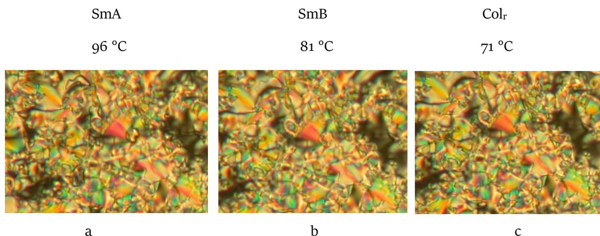
**Figure 4.3** Polarised microscopy views of the different mesophases of compound [M-2]-C.
