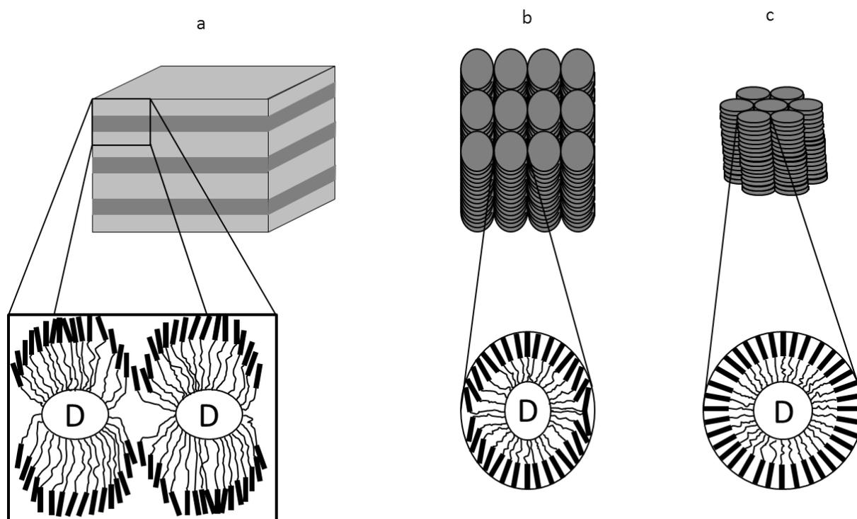
**Figure 1.17** Structure of mesophases at different generations (D: dendritic part, further explanation in the text)
