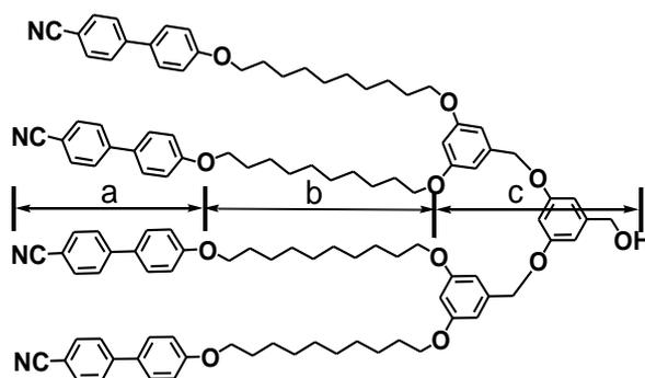
**Figure 4.1** Example of intramolecular distance determination. The sum of the sequential values gave the length. a (terminal N of the cyano-group – O at the other end of the biphenyl) = 1.10 nm, b (the two oxygens at the ends of the decamethylene chain) = 1.36 nm, c („starting” O of the dendritic scaffold – H of the focal OH) = 0.98 nm.
