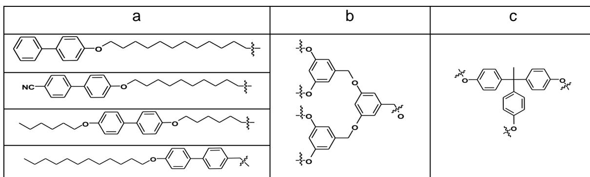
**Figure 2.1** Target liquid crystalline dendrimers a, end-groups, b, dendritic scaffold, c, central core unit
