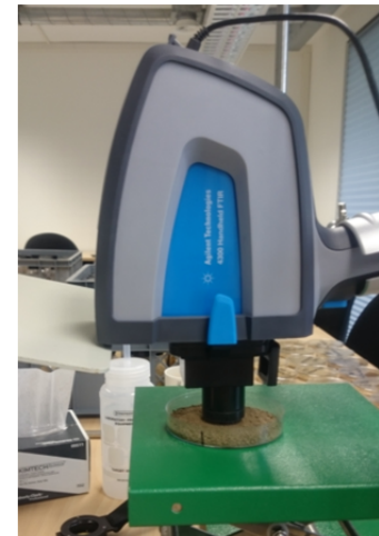
Fig. 4.6: Spectral measurements with the Agilent 4300 Handheld FTIR.
