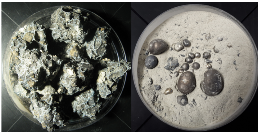
Fig. 2.9: Left: Fresh AOD converter reduction slag with metal granules. Right: Self-pulverisation of the sample due to dicalcium silicate decomposition leaving only the formerly embedded granulated metal shots.
