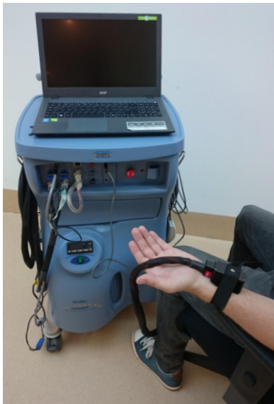
Figure 5.1: MR compatible thermode placed on the left forearm and control unit.
