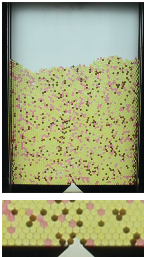
Fig. 1 Top: Image of the container filled with a mixture with 10% hard frictional beads. Yellow and pink colored hydrogel spheres are equivalent, airsoft bullets appear dark. Bottom: Zoom into the region near the orifice at the bottom, in a clogged state. The orifice in these images is D = 11 \text{ mm} , slightly less than two particle diameters.
