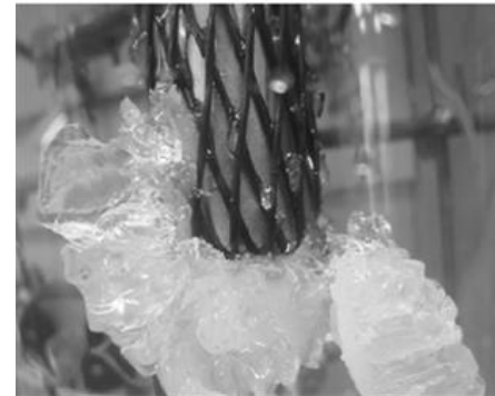
Figure 4.6. Cold finger with grid and parts of burst crystal layer. Crystal layer was grown from a complete seed layer in a melt containing glycerol and w_w = 3\% water at T_B = 15^\circ\text{C} and T_{CF} decreasing exponentially from T_{CF}(t = 0) = 5^\circ\text{C} to T_{CF}(t = 60\text{ h}) = -10^\circ\text{C} . After draining of the melt, sweating was started at T_B = T_{CF} = 15^\circ\text{C} until layer burst.
