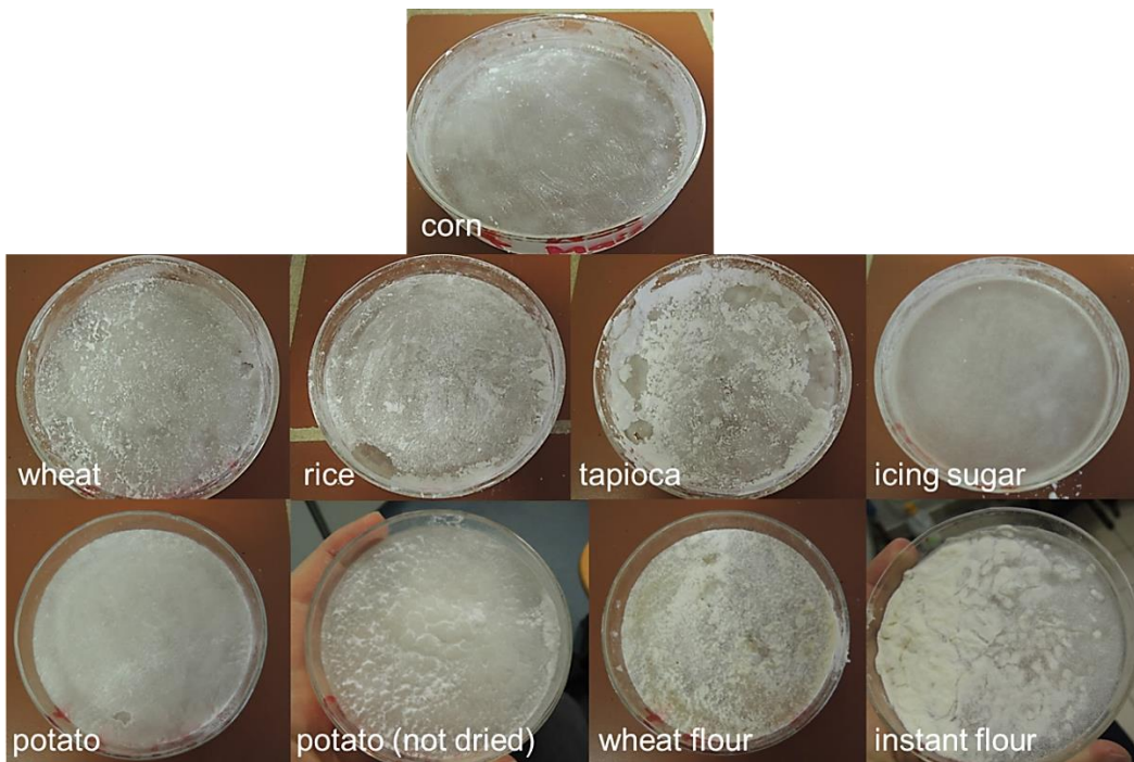
Figure 5.5-13: Crystallization in petri dishes ( d \approx 11.0 - 11.5 cm) with different seeds, at 50 °C [Kat16]
