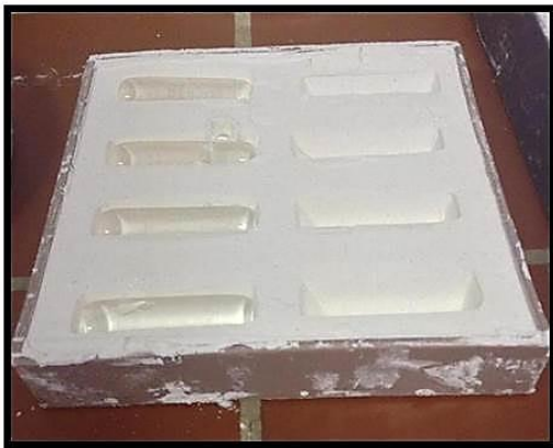
Figure 4.1-3: Corn starch mold with imprints filled with sugar solution [Her16]
