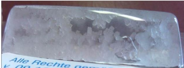
Figure 5.5-1: Crystallization in the absence of seed materials in a 1.0 wt% agar-sugar solution [Her16]
