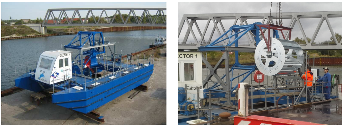
Figure 3.7: Photos of the Vector 1 research catamaran. Left, the berthed boat; Right, installation of the mid-size free-stream waterwheel using a crane.
