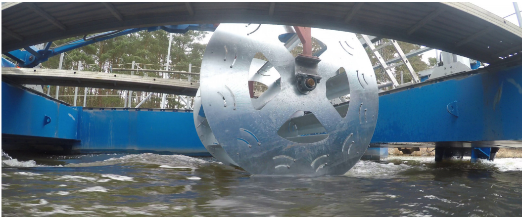
Figure 3.10: Still from a video recording carried out using an action camera during the experiment campaign. The camera is hoisted on the boat's port hull, pointing starboard; the flow relative to the wheel is from left to right in this image. In this case, the velocity is 2.1 \text{ m s}^{-1} . A large-amplitude stationary wave is visible immediately ahead of the wheel, while the wheel itself is operating in the stationary trough that follows the wave.
