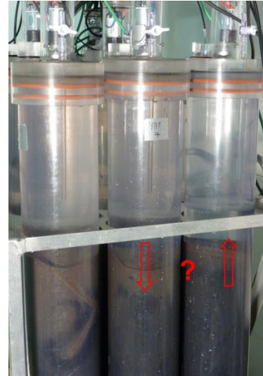
Image: Hassel shallow site sediment cores at the end of incubation, showing a chironomid burrow (left core). Image by Tallent Dadi
