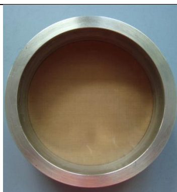
Metallic plate covered with polytetrafluoroethylene film.
