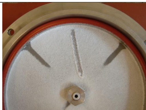
Accumulation of film particles inside the coating device.
