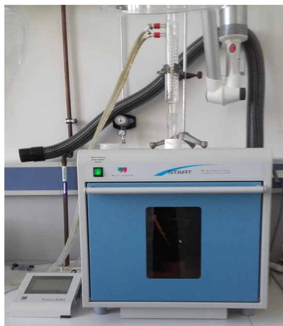
Figure 2.1: START 1500 Microwave reactor.
