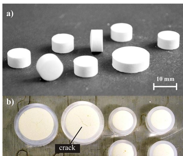
Fig. 5.2-18: Images of produced paracetamol tablets (a) and crack-like behavior (b) [Ngu15b].
