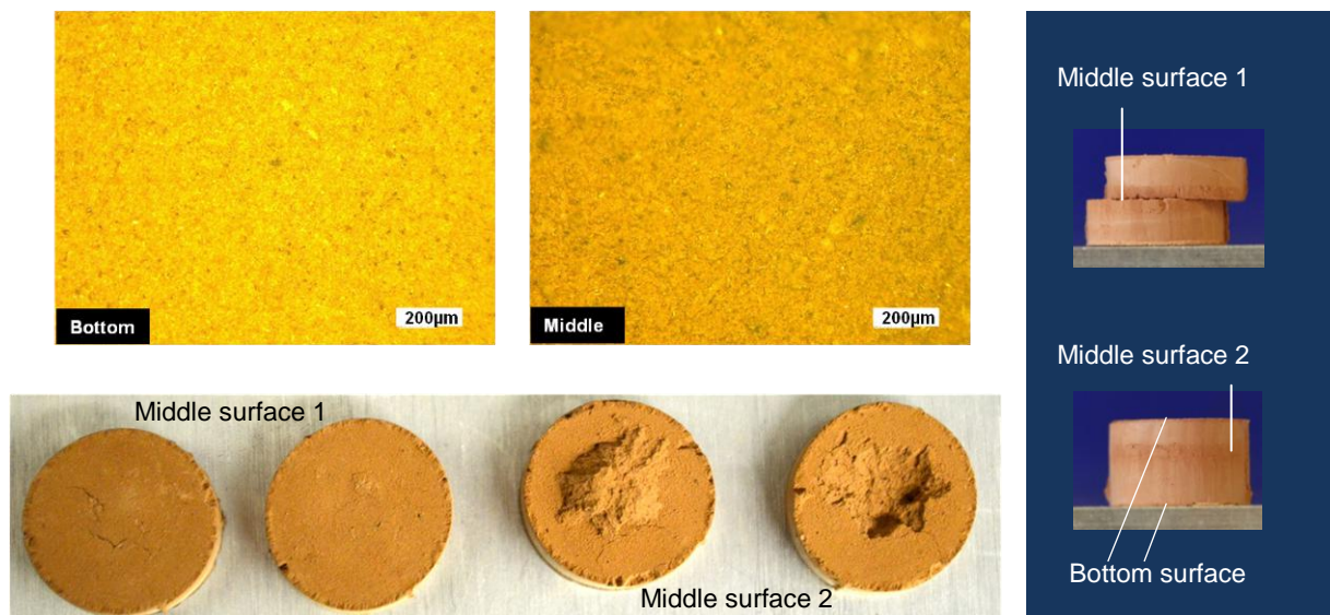
Fig. 5.1-20: The view of the bottom surfaces and the middle surfaces of middle-broken tablets.
