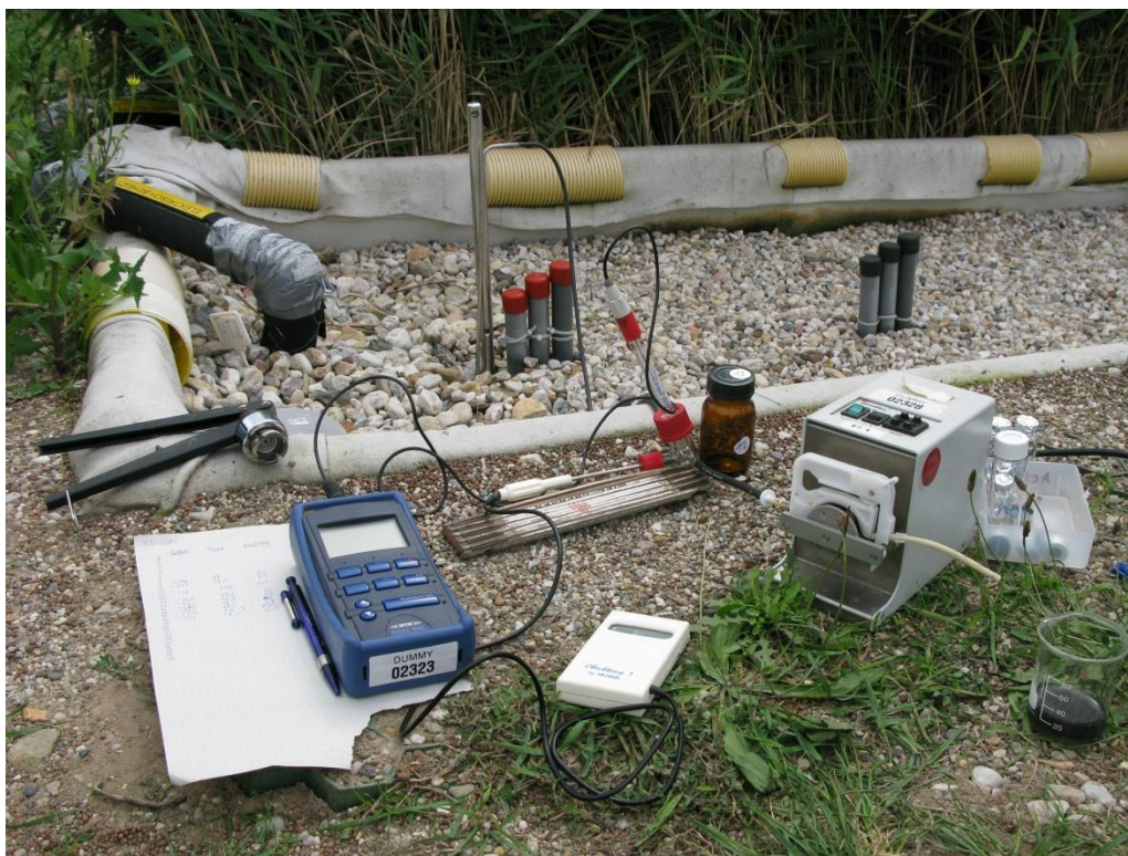
Figure 6 Instruments used for the pore water sampling (still lance, sensor probes and peristaltic pump. The picture was taken by the LRB-Team).
