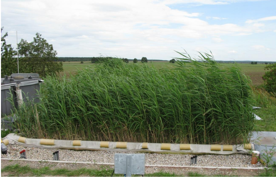
Figure 4 Spatial preferential growth of the plants along the water flow path (from left to right) in a HSSFCW.
