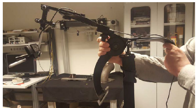
Fig. 7 Construction for a body-worn camera to ensure the permanent analysis of subjects facial expressions
