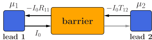
Figure 4.2: The two-terminal scheme for measuring the tunneling conductance of a barrier between two ideal leads in one-dimensional case.
