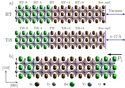
Figure 5.1: The side view of the supercell with vacuum (a) and without vacuum, i.e. superlattice (b), both of which were used to model the \text{BaTiO}_3/\text{SrTiO}_3 (001) interface. The two different terminations, \text{SrO}/\text{TiO}_2 and \text{TcO}_2/\text{BaO} , are marked as TiS and BT, respectively. The numeration of atomic layers outward the interface, as shown in the panel (a), is used throughout all further figures and text. The electric polarization of \text{BaTiO}_3 is oriented along the [001] direction (shown by the horizontal arrow).
