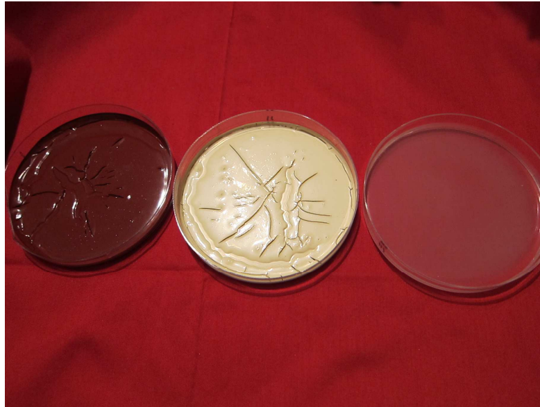
Figure 5.9: Surfaces of various water-based lacquers inside Petri dishes with a diameter of 9.6 cm (WGR, WGI, WGC each 15 g)
