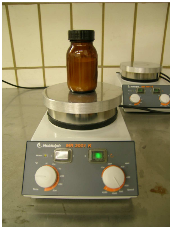
Figure 3.14: Lacquer mixture inside a 100 ml amber screw cap bottle on a magnetic stirrer
