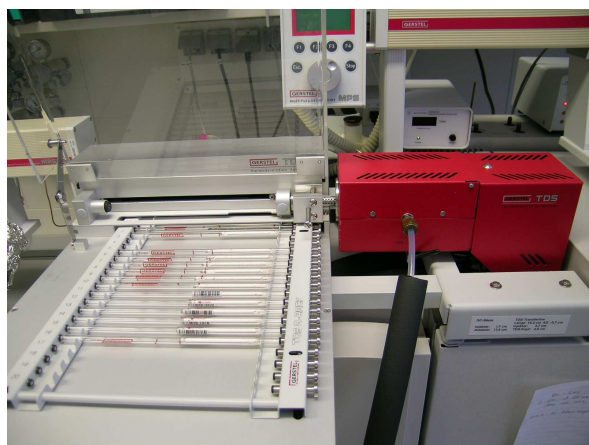
Figure 3.9: TDSA with glass sampling tubes inside the autosampler (GERSTEL)
