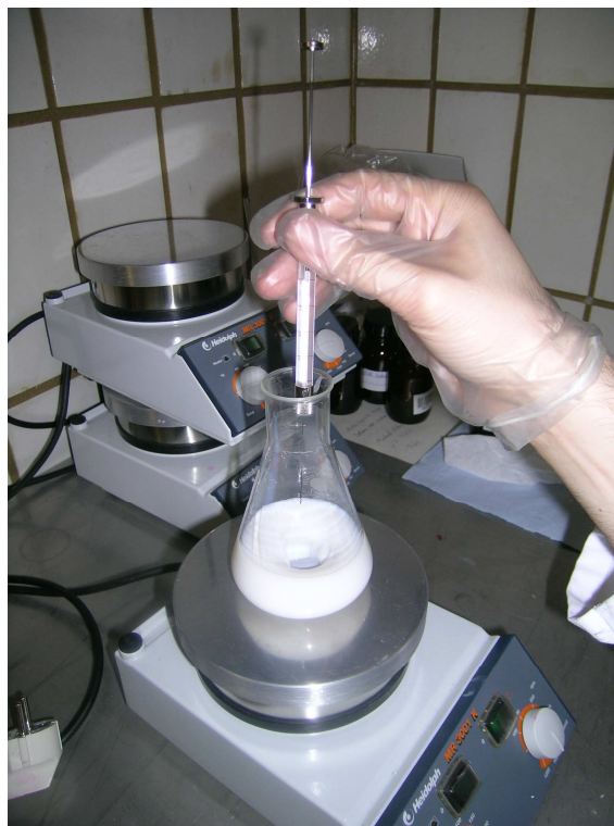
Figure 3.15: Addition of the pure analyte into the agitated lacquer with a glass syringe
