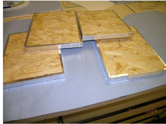
Figure 2.5: Oriented strand boards with sealed cutting edges
