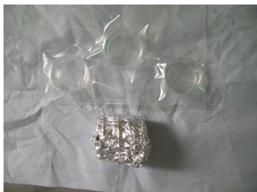
Figure 4.17: Lacquer samples vacuumed in a LDPE bag (on top) and packed in aluminium foil (below)
