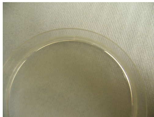
Figure 5.24: Plane surface of a cured lacquer mixture without containing MeOH
