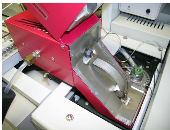
Figure 3.10: Transfer line of the TDSA (GERSTEL)
