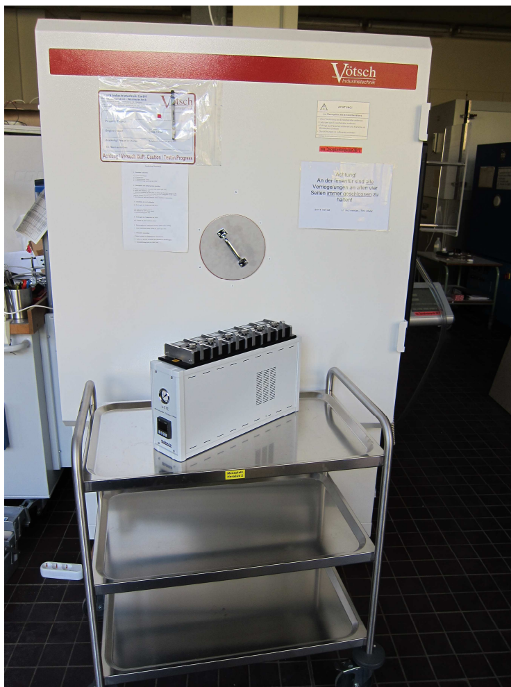
Figure 4.2: Size-comparison of a micro-chamber (front) in opposite of a 1-m 3 -chamber (back)
