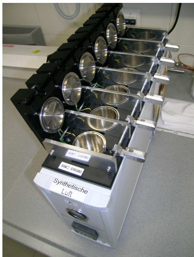
Figure 3.4: Micro-Chamber/Thermal Extractor™ ( \mu -CTE™) from MARKES Int. (opened)
