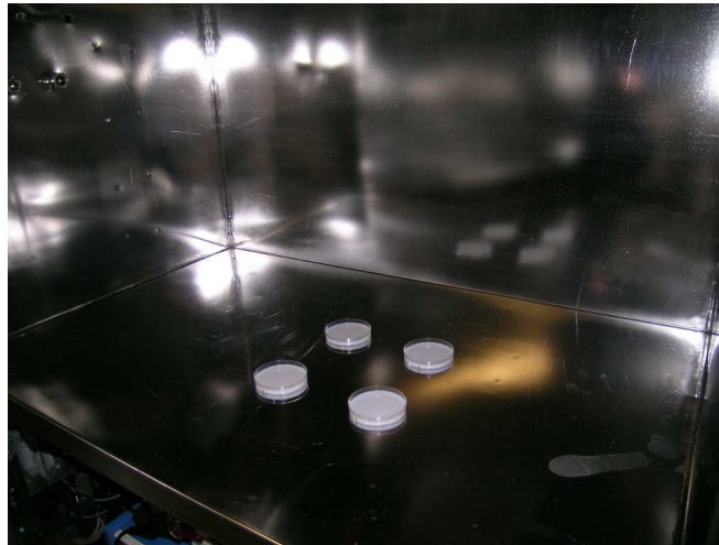
Figure 4.9: Lacquer samples loaded into a 1-m 3 -chamber for curing
