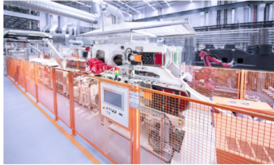
Figure 12: Calendar-Direct Impregnation Machinery system in OHLF lab
