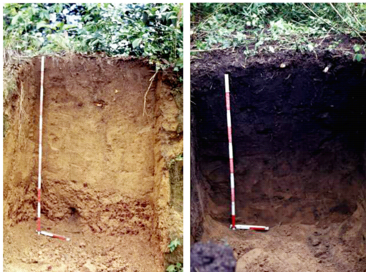
Figure 2.1 Left: Typical Ferralsol profile. The shallow surface horizon is light brown coloured and roots are concentrated at the soil surface. Below this horizon follows a thin transition horizon to a subsoil horizon which can be several meters thick. The texture of these soils is loamy or sandy and the structure is dominated by stable micro aggregates (pseudo-sand). Right: typical terra preta profile. The topsoil horizons are dark grey or black coloured and can reach a depth of more than 1 m. Potsherds, small bone and charcoal particles are characteristic for this horizon. Roots reach deeper down in higher density than in Ferralsols and signs of bioturbation and aggregates of biogenic origin can be found frequently. Below follow transition horizons which are lighter coloured and typically show patches of different brown, grey and black colours with clear signs of mixing of topsoil and subsoil material. The subsoil horizons are identical to the subsoil horizons of adjacent soils. Terras pretas typically have the same texture like surrounding soils (from Glaser et al., 2001b).
