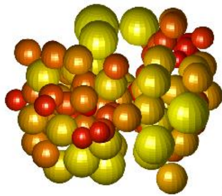
Figure 5. An exemplary agglomerate (with N_p = 100 ; red for the smallest (122 \mu\text{m} ) and yellow for the largest (396 \mu\text{m} ) primary particle) generated using the MPTSA model (with R_p = 260 \mu\text{m} and \sigma = 52 \mu\text{m} ).
