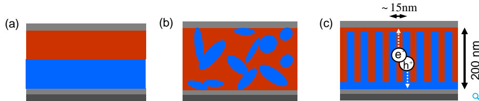
Figure 1.1: Schematic representation of donor-acceptor morphologies of organic solar cells (a) bilayer morphology, (b) phase separated donor-acceptor blend morphology and (c) ideal heterojunction morphology. The donor component is shown as blue while the acceptor component is shown as red.
