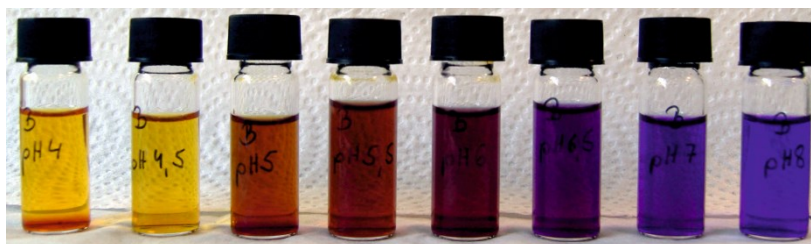
Figure 34 Colour gradients of pH indicator dye bromocresol purple in buffers of different pH.
