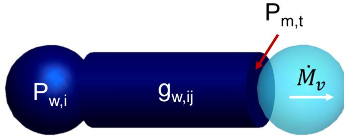
Figure 2.10: Liquid pressure demand of stationary meniscus. The dark blue color represents the liquid, and the light blue color represents the vapor.
