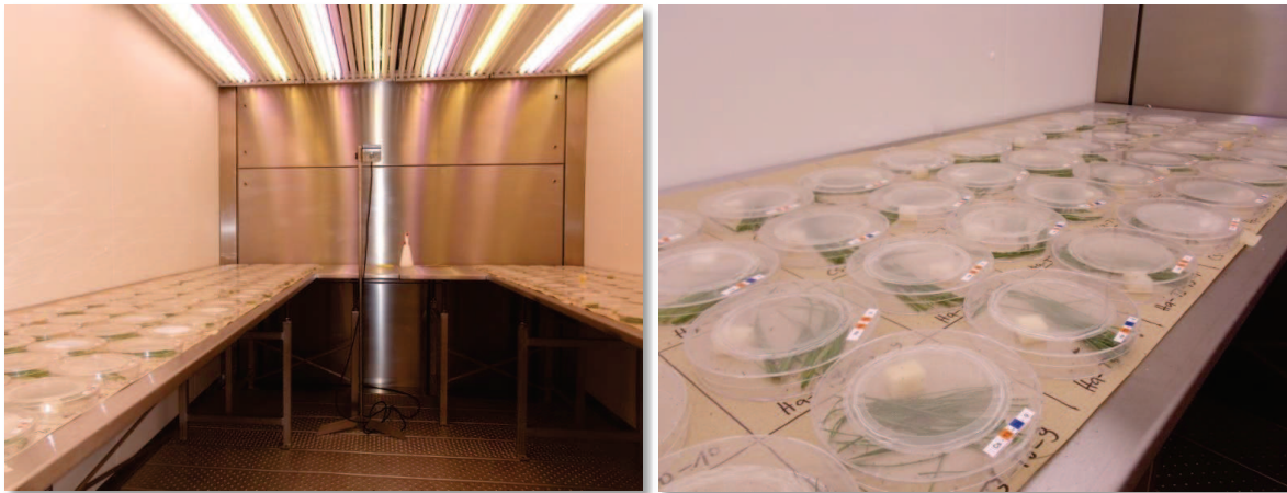
Figure 10: TIRA BIO TB 818.1 climate chambers (TIRA Umweltsimulation, Schalkau, Germany) equipped with experimental petri dishes (pictures by Sandra Krenzel)
