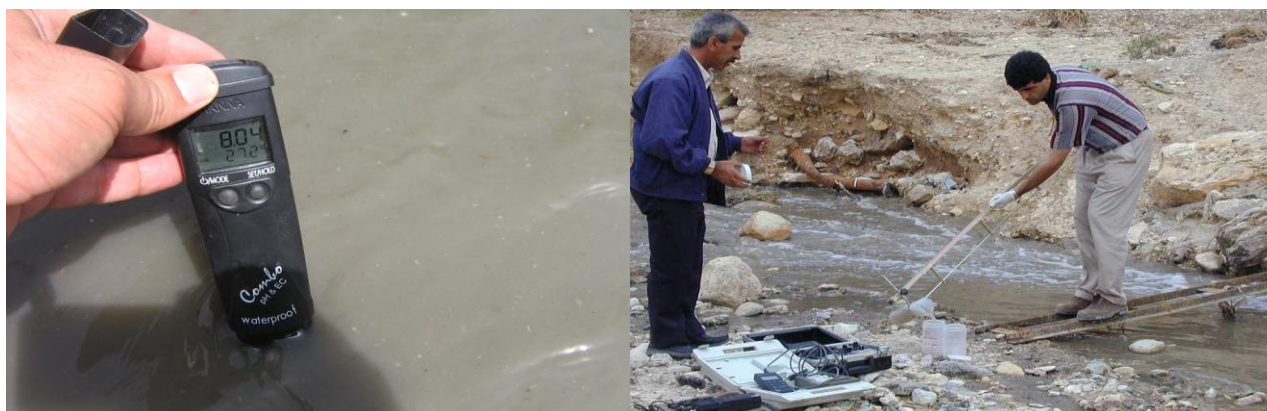
Figure 2.10: Measuring physical parameters in the left (pH, Temperature and TDS) and in the right the dissolve oxygen at Al-Qilt catchment.
