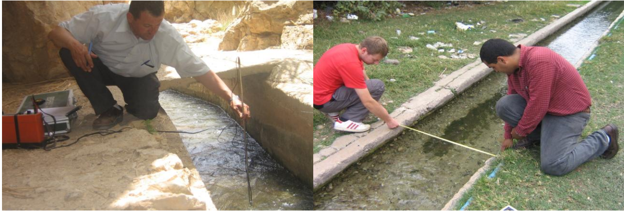
Figure 2.9: Measuring the discharge using the current meter at Al-Qilt catchment.
