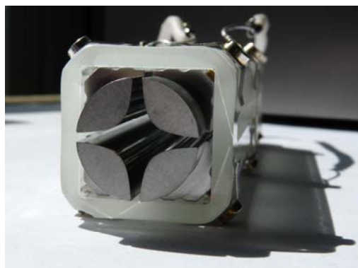
Figure 12: Scheme of a linear quadrupole mass analyzer with cylindrical rods (left) and image of a quadrupole from a Thermo Finnigan TSQ 700 triple quadrupole mass spectrometer with hyperbolic rods (right).
