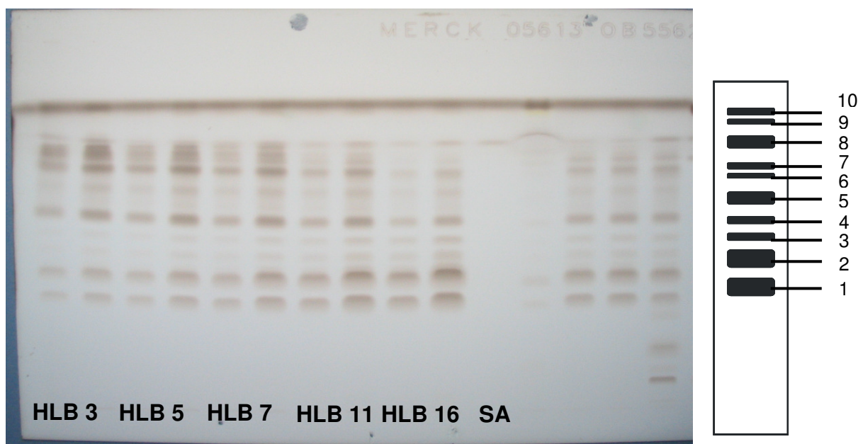
Figure 26 Photograph of a HPTLC plate after separation via a 4-step development program based on methanol/water/chloroform and post-chromatographic derivatisation. Five sucrose ester (SE) preparations ranging from HLB 3 to 16 and stearic acid (SA) were spotted onto the silica plate representing 50 and 125 \mu\text{g} of the SE, respectively. The different SEs were separated into 10 fractions as illustrated in the drawing to the right. Less polar SEs reflected by lower HLB values contain higher amounts of sucrose polyesters and less amounts of mono- or diesters. For polar SEs with high HLB values this effect is vice versa. For SE with an HLB of 3 the intensity of spots 8-9 is higher in comparison to the polar SE with HLB 16. For the polar SE with HLB 16, the intensity of spots 1-4 is much higher in comparison to the SE with lower HLB values.
