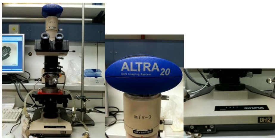
Figure 3.2.2.1: Light microscope Olympus BH2, an Olympus ocular NFK 2.5x LD 125 and an objective of IC 5 (MDPlan5 / 0.1), digital camera ALTRA 20.
