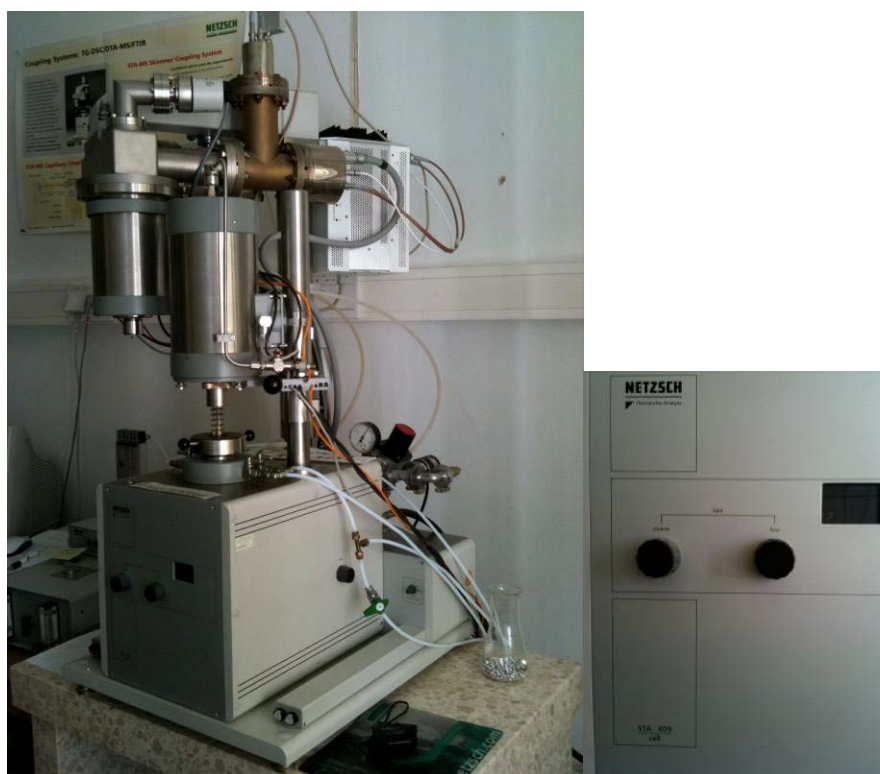
Figure 3.2.2.6: Coupling system of Netzsch TG–DSC/DTA (STA) with Netzsch STA 409 cell.
