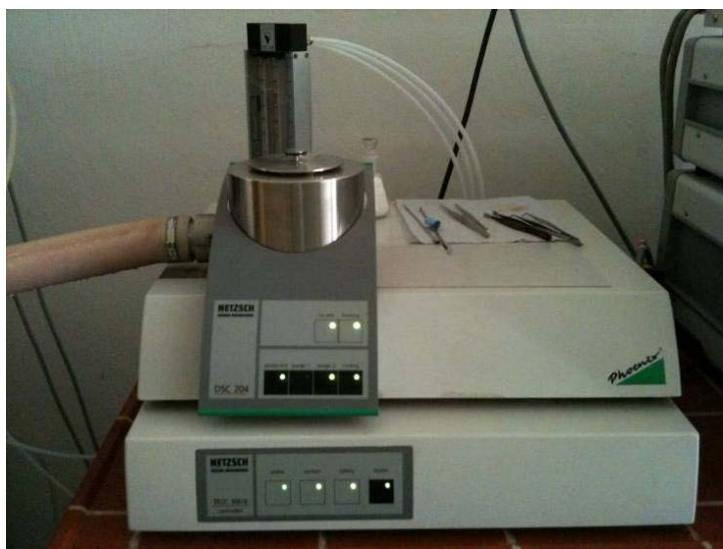
Figure 3.2.2.5: Differential Scanning Calorimeter (DSC) Netzsch DSC 204, Netzsch TASC 414/4 controller.
