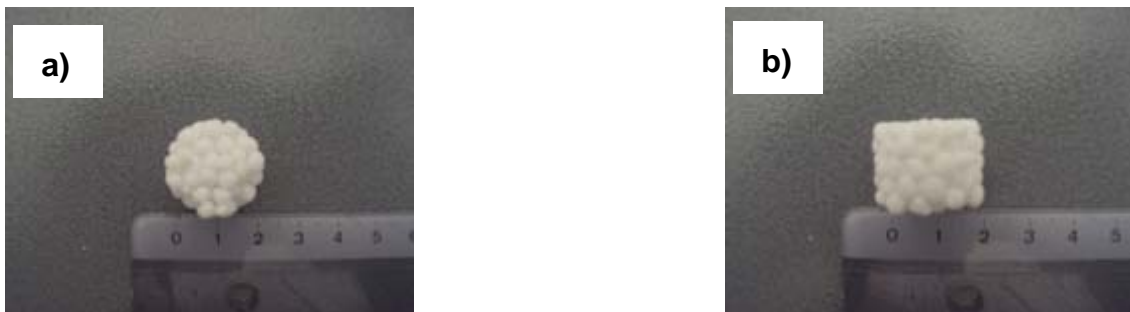
Figure 3.10: Top view of caked granules (a) and side view of caked granules from MPS (b).
