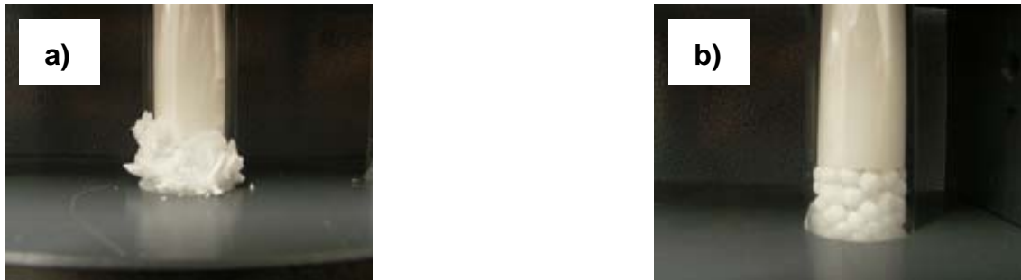
Figure 3.9: Granules coated with F8-coating solution (a) and T8-coating solution (b) in MPS.
