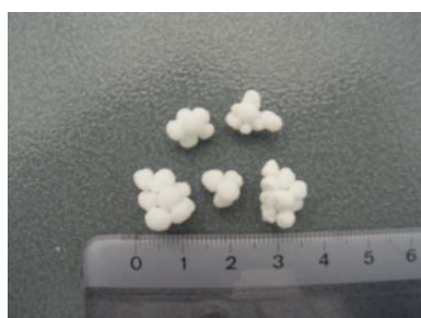
Figure 3.11: Still caked granules after falling from 1 m height (only single granule was)
