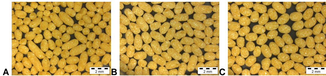
Figure 54. Spheres after pelletization and spheronization using the pelletizing methods oscillating sieve (a), ball mill (b) and the simulating pelletizer (c). Containing SE S-1170 80 %, total vitamins 5 % and tricalcium phosphate 15 %.
