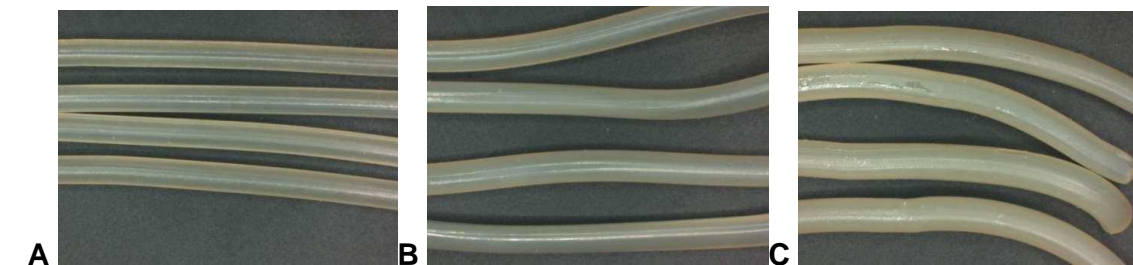
Figure 46.A. Pictures of SE S-1170 strands extruded with a screw speed of 4 rpm at 50 °C (A), 55 °C (B) and 60 °C (C).
