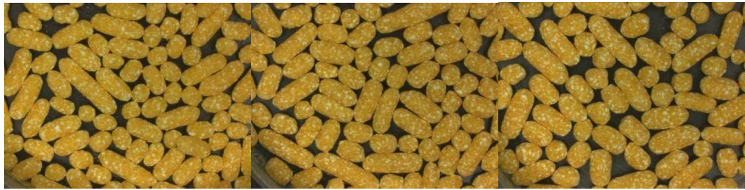
Figure 43.A. Pellet formulations containing 80% SE S-370 (A), S-770 (B) and S-1170 (C), 15% MCC 5% vitamins. Spheronization parameters: 1000 rpm, 10min.
