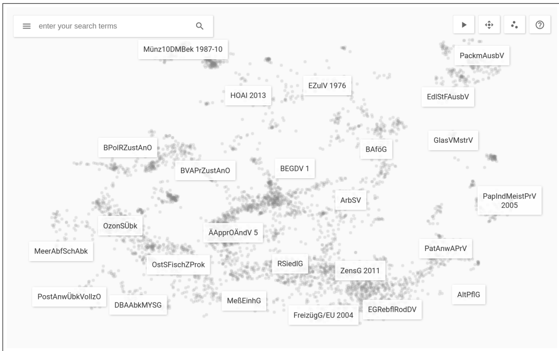
Figure 45: User Interface Prototype showing a map of German laws: each disc corresponds to one document; boxes with law abbreviations can be clicked to open a law, or moved to begin personalization phase; when entering a search query, results will be highlighted, see Figure 46; users may zoom into the map using touch gestures or mouse scroll.
