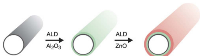
FIG. 1. (Color online) Schematic view of the fabrication process of CNTs covered by a thin \text{Al}_2\text{O}_3 layer and subsequently by a layer of ZnO (type B tube). The thickness of the ZnO and the \text{Al}_2\text{O}_3 shell is controlled by the number of ALD cycles.
