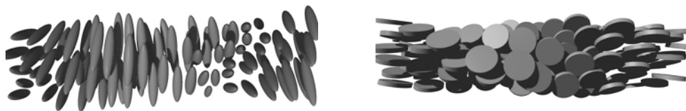
Figure 1.8: Cartoons of the helical director modulation in the chiral nematic (or cholesteric) phase for the case of rod- and disc-shaped building blocks, respectively. Each rod or disc represents either a mesogen (thermotropics) or micelle (lyotropics) with the corresponding shape. Note that, for clarity, the pitch has been drawn orders of magnitude smaller than in reality and the local degree of order is much too high.
