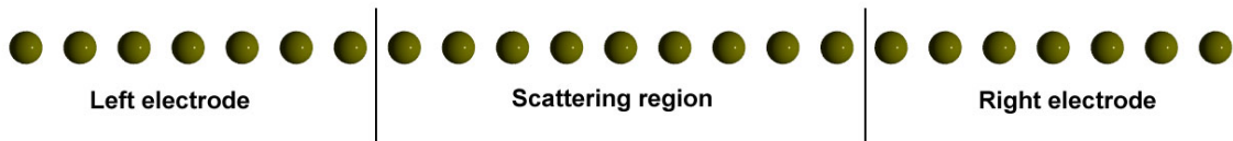
Figure 5.5: Schematic structure diagram for the transport calculation through the monoatomic iron chain.
