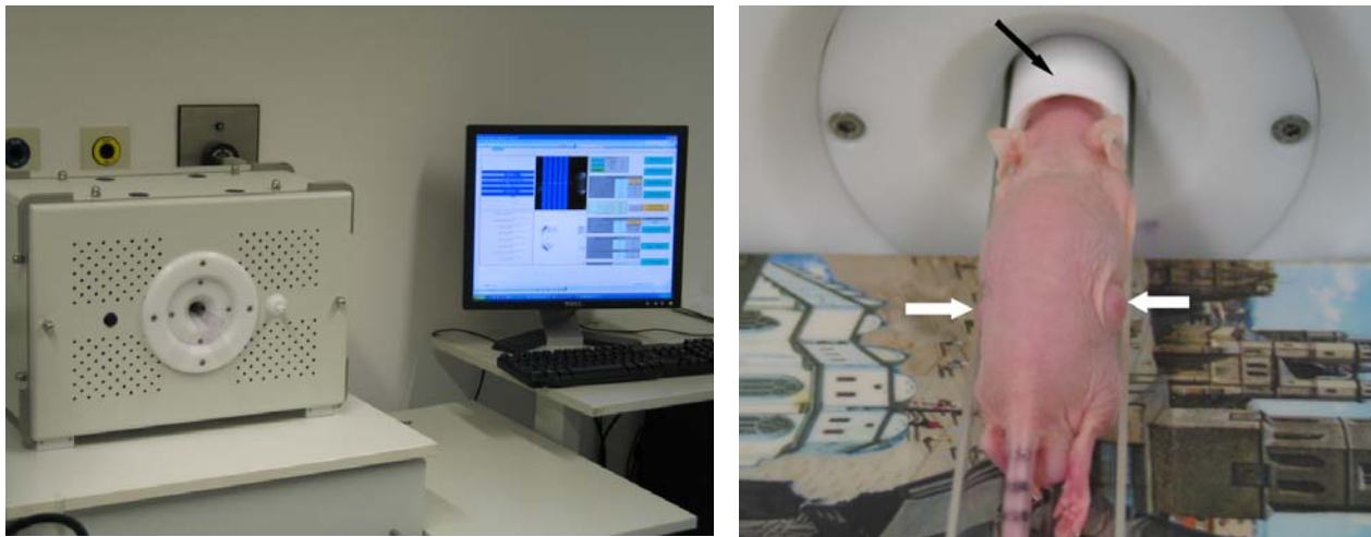
Figure 5.5. The left photograph shows the Benchtop MRI spectrometer for in vivo imaging from Oxford Instruments, UK, while the right one shows an anaesthetized nude mouse with anaesthesia mask (black arrow) and subcutaneously-injected tumors (white arrows).
