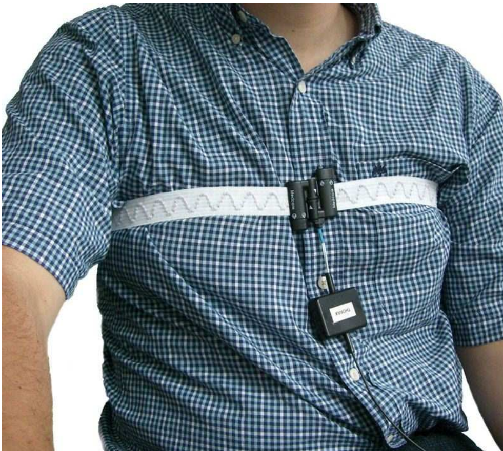
Figure 12: Becker Meditec Respiration Belt For measuring chest respiration, as used in the experiment.
