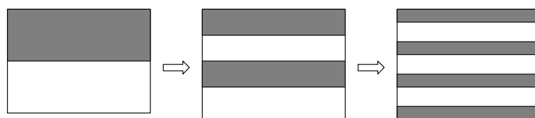
Figure 3-3. Schematic representation of distributing mixing in laminar flow [72]
