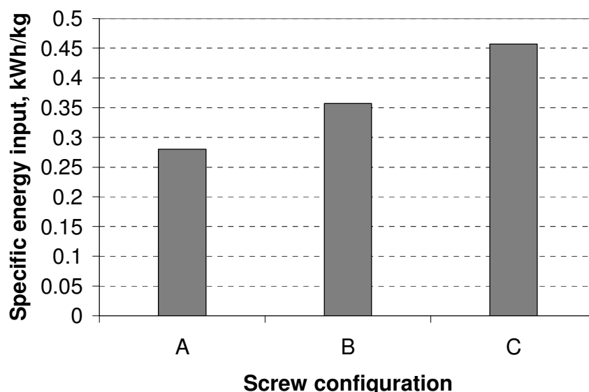
Figure 5-3. Specific energy input of the extrusion process using screw configurations A, B and C
