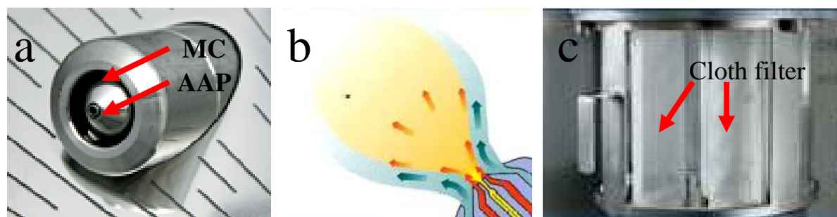
Figure 5-4: Picture (a) and schematic view (b) of three component nozzle (spray liquid in yellow, AAP in red and MC in blue) and cloth filters in the spray dome (c). Figures adapted from [14, 72].
