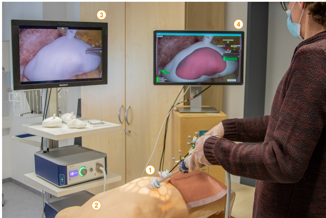
Figure 6.5: Overall study setup. The laparoscopic tools are inserted in the trocar ports (1) of the torso model (2). The left screen (3) displays the unaltered laparoscopic video. The right screen (4) is currently showing the InstControl GUI. The optical tracking camera is to the top left, outside the photograph's field of view and the mouse is located behind the torso model (to the user's right).
