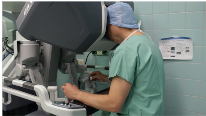
(a) Surgeon console of the da Vinci robot. Image courtesy of Prof. Martin Schostak, University Hospital Magdeburg.
