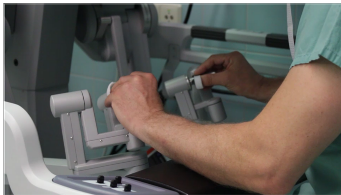
(b) Instrument controllers of the da Vinci robot. Image courtesy of Prof. Martin Schostak, University Hospital Magdeburg.
