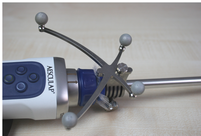
(b) Passive infrared tracking markers on a unique geometry marker shield (Cascination AG, Bern, Switzerland). The marker shield is mounted to a laparoscopic camera head.
