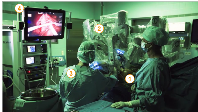
(c) Bedside view of the da Vinci robot during surgery, including the patient (1), the bedside cart with the robot arms (2), the bedside assistant (3), and the assistants' view of the laparoscopic video stream (4). Image courtesy of Prof. Martin Schostak, University Hospital Magdeburg.
