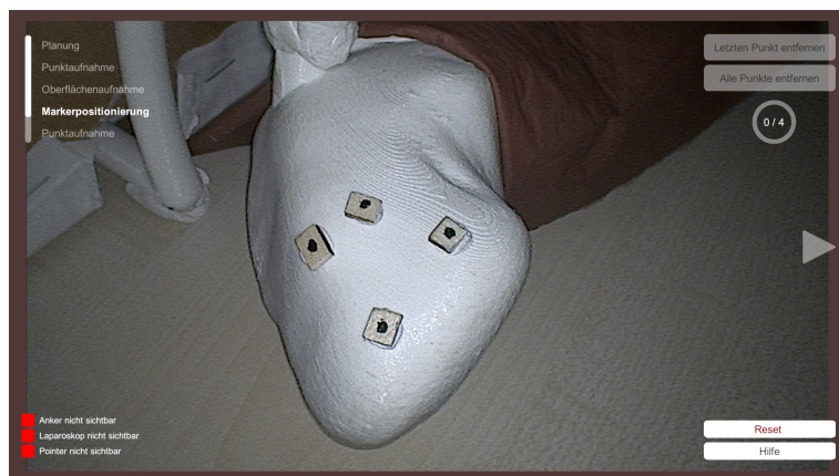
(c) Partially occluded phantom with the simulated adhesive markers. The image also shows the GUI that is displayed while the user first records the marker positions.
