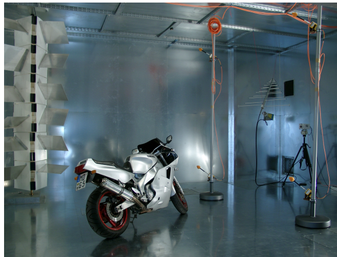
Figure 2.12: Photograph of the big reverberation chamber at the at OvGU [Wik20]
