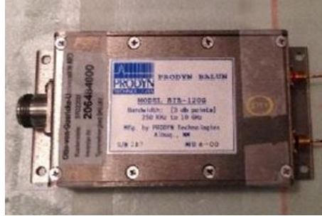
Figure 5.27: Balancing unit for the measurements with three wires
