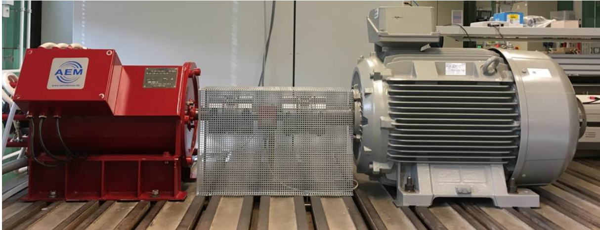
Figure 3.8: Traction (left) and Load machine (right) in the test bench.
