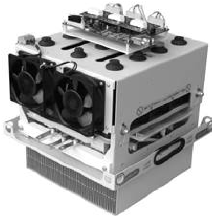
Figure 3.9: Inverter for the drive of traction and load machine.
